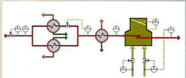
In the case shown in TOPAS (see diagram) the temperature can be increased by almost 3 degrees. At the current prices for energy (crude oil 80 US\$/bbl) savings of 500 € per year, m<sup>3</sup>/h product flow and degree C temperature increase can be realized.
