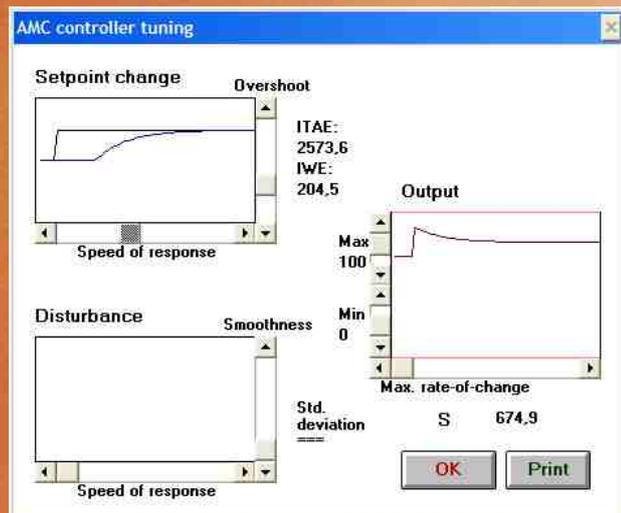
Users can specify the desired performance: Faster or slower, without or with some overshoot and also constraints on the manipulated variable. The so achieved performance is shown on the screen and the results can be tested with the integrated simulation environment in TOPAS.
