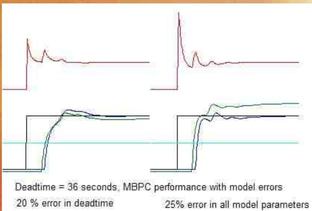
In the tests on the left, the AMC controller uses an imperfect model, first with an error in the dead-time and then with 25% error in all process parameters. It cannot work so smoothly any more but is far from poor performance or even instability.
